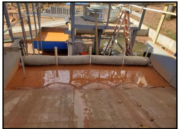
Ponding and Sediment Build-up Behind Product at end of Flow (30 minutes) and at end of Seepage (75 minutes)
