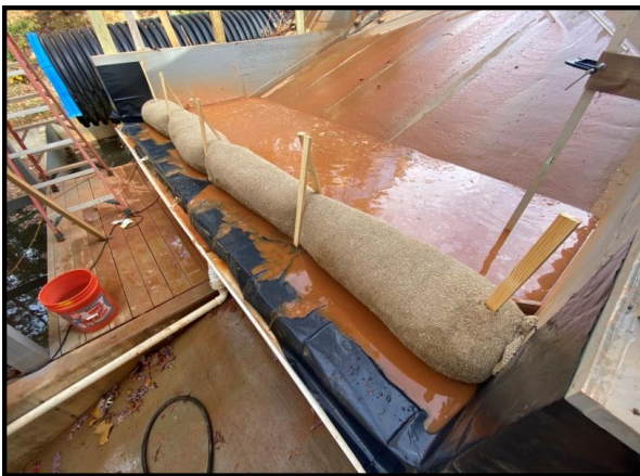
Ponding and Sediment Build-up Behind Product at end of Flow (30 minutes) and at end of Seepage (75 minutes)
